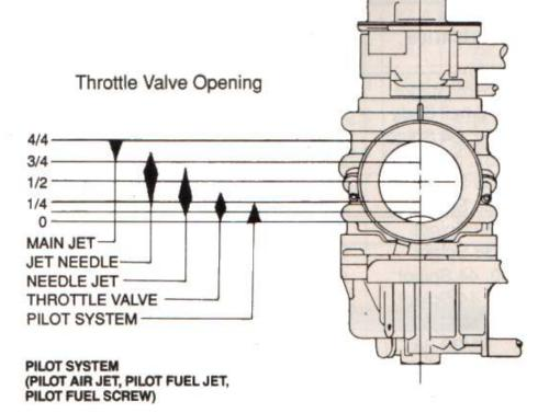
THIS IS A BRIEF EXPLANATION OF WHAT CONTROLS WHAT IN YOUR CARBURETOR. OBVIOUSLY GOING WITH A LARGER JET ON ANY OF THESE WILL MAKE THAT CIRCUIT RICHER AND GOING SMALLER WOULD LEAN THAT CIRCUIT OUT.
